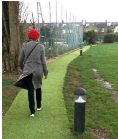
Photo 9: Artificial grass path from Main Clubhouse to SE area & Turney Road pedestrian entrance. Bollard-mounted down lights illuminate path at night whilst controlling light spillage. Existing 4m high protective netting can be seen in the background. A wider path would improve access.
